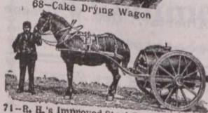
71—R. H.'s Improved Steel Tank Cart. 300 Gallons capacity
