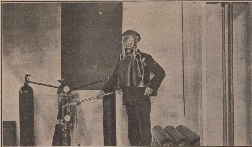
Another corner of Rescue Station, showing refill pump, portion of exercising device and 6 oxygen cylinders.
