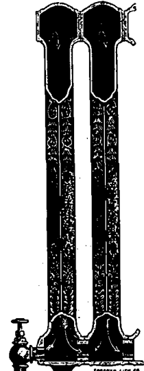
Sectional View of Steam Radiator Showing Form of Connection.
