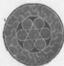
Locked Coil Aerial Cable or Colliery Guide.
