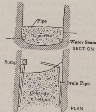
Fig. 5. Second Method of Handling Water in Core-Wall Ditch.
