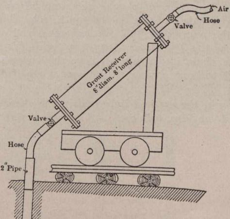
Fig. 2. Grouting Device Tried and Abandoned
