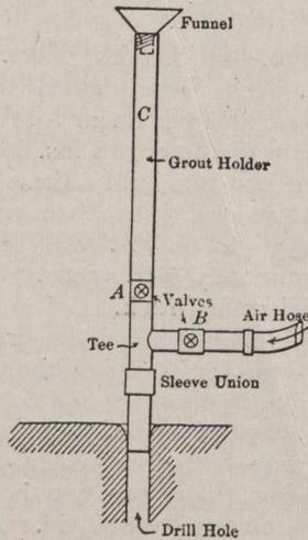
Fig. 3. Grouting Device Employed.
