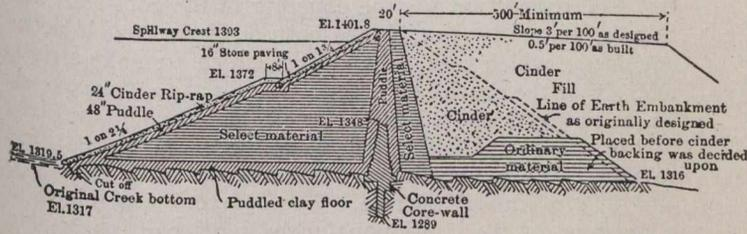
Fig. 1. Maximum Cross Section of Hinckston Run Dam.
