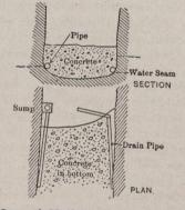
Fig. 5. Second Method of Handling Water in Core-Wall Ditch.
