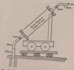
Fig. 2. Grouting Device Tried and Abandoned
