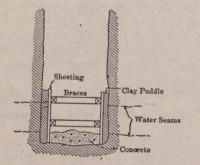
Fig. 4. First Method of Handling Water in Core-Wall Ditch.
