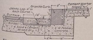
Fig. 2.-Granite Curb and Vitrified Brick Gutter.
