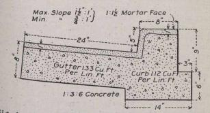
Fig. 1.-Standard Type of Combined Curb and Gutter.
