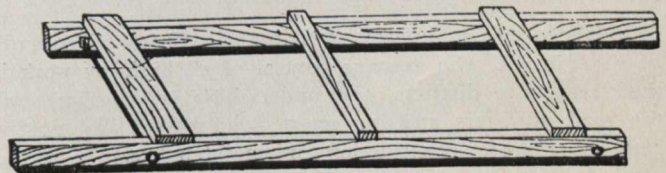
Modification of Split Log Drag—Made of Timbers.
