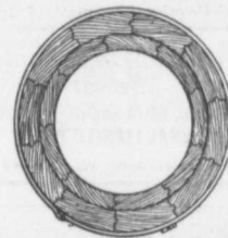
End view of Pipe and Coupling.
