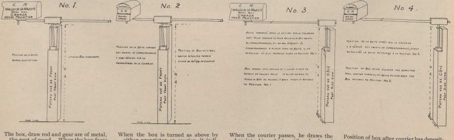
The box, draw rod and gear are of metal, the post of wood. When the box faces as shown, it indicates to both proprietor and courier that the box is empty.
