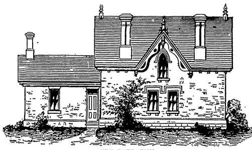
The extreme outside dimensions of this house are | bedrooms, the stair rails, newels, and balusters, 24 feet wide, 32 feet long; the kitchen extension is 15 feet wide, and 19 feet long.
