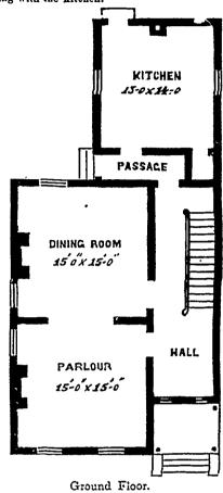
The cellar, which should have a concrete floor, and be well drained and ventilated, is under the dining room, and the stairs leading to it are under the main stairs.
