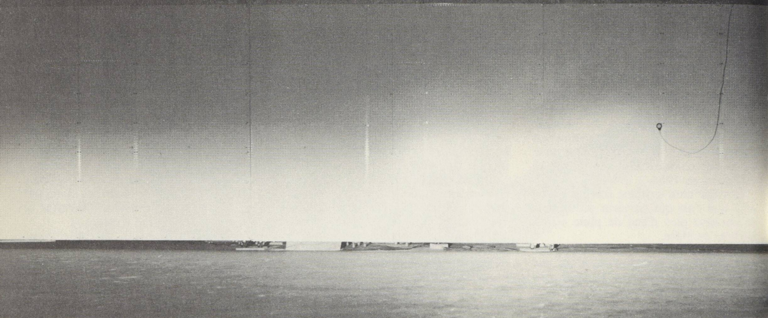
Photograph of light distribution of an SAE standard headlight in the passing mode. Note lack of definition on left hand side.
