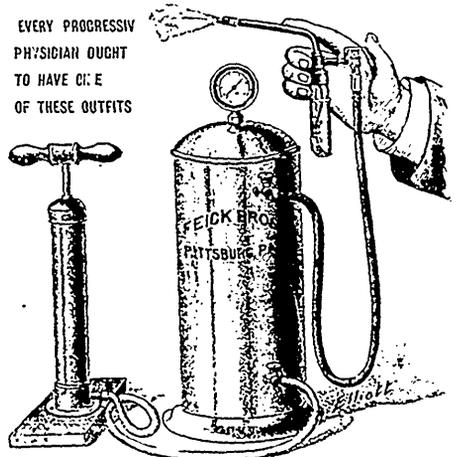
The receiver is 27 inches high, including gauge, and 10½ inches in diameter; tested to 100 lbs. hydraulic pressure, and provided with a gauge registering the maximum pressure of 50 lbs. Both receiver and pump are made of copper and are nickel-plated. Complete outfit consists of improved pump, silk tubing, automatic cut-off, and three Davidson hard-rubber sprays, or glass sprays.
