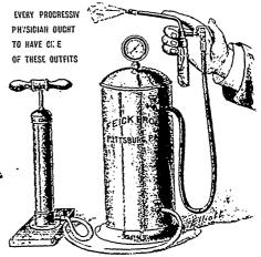
The receiver is 27 inches high, including gauge, and 101 inches in diameter; tested to 100 lbs. hydraulic pressure, and provided with a gauge registering the maximum pressure of 50 lbs. Both receiver and pump are made of copper and are nickel-plated. Complete outfit consists of improved pump, silk tubing, automatic cutoff, and three Davidson hard-rubber sprays, or glass sprays.
