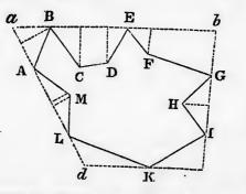
When there are obstructions within the figure, such as wood, water, hills, &c., measure the lengths and positions of the four-sided figure  $a \ b \ c \ d$ , taking care to measure the offsets from the different corners as you go along. gro two by the fro con of sur
