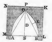
1. What is the content of a concavity of a semi-circular vaulted roof, the span being 30 feet, and the length of the vault 150 feet?
