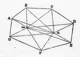
Let m and n be two stations, from which all the marks A, B, C, &c., can be seen, plant the instrument at m and by it, measure the angles A m n, B m n, C m n, &c. Next measure m n, and planting the instrument at n, measure the angles A n m, B n m, C n m, &c. These observations being planned the lines joining the points of external intersection, will give a true map of the ground. The method of finding the content will be shown further on.
