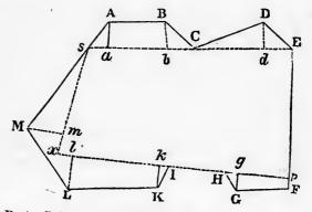
s C B A, C D E, &c. must be added to the area of the quadralateral s x F E. But when the principal lines are taken outside the figure, the portions included between them and the boundaries of the field are to be deducted from the content of the quadralateral, and the remainder will give the true content of the field.
