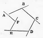
the angle A; next measure A B, and planting the instrument at B, measure, as before, the angle B; measure the line B C, and the angle C: and so proceed round the figure, always measuring the side as you go along, as also the
