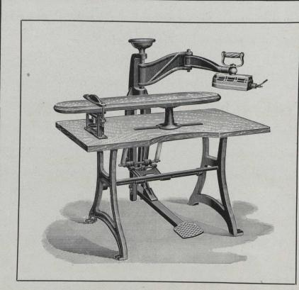
THE BUSKARD NO. 4. A quick action pressing machine, light and easy to handle, and has a pressure on the iron of 250 lbs.
