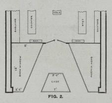
As in the case of buildings treated in our previous article, the walls in the plans here submitted are designed to measure 18 inches wide; hence, it is readily seen that if the walls of a building are only 12 inches wide, another foot can be added to the available width of the store, which can be utilized for additional width to the CLOTHIER AND HABERDASHER, JULY, 1910. windows or vestibule. This additional foot is also available for widening the main aisle to that extent.
