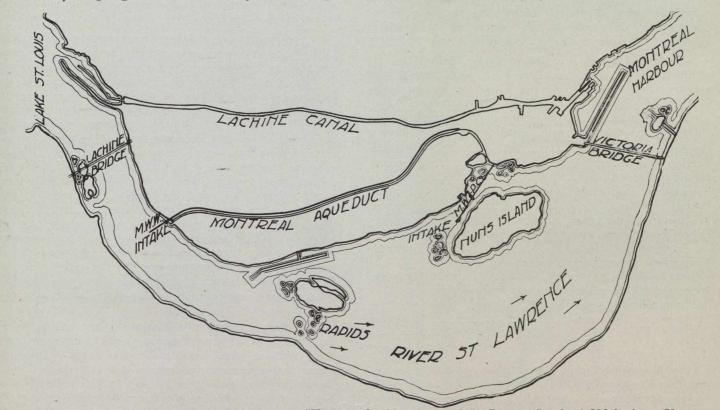
Fig. 1.-Part of Montreal Island, Showing the Waterworks Aqueduct and the Present Intake 1,200 ft. from Shore.
