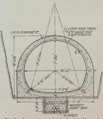
Fig. 2.—Cross-section of Intake Conduit, Montreal Waterworks.
