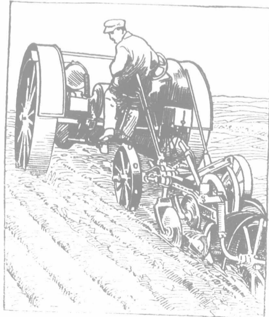
Happy Farmer Tractor handling 3 bottom 14 inch plow back-setting Timothy Sod
