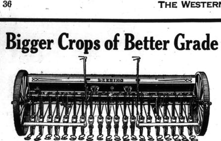
**B**IGGER CROPS and a better grade of grain result from planting with **DEERING** drills. They plant the seed at a uniform planting with **DEERING** drills. They plant the seed at a uniform depth, giving the whole crop an even start and producing an even stand. Even ripening, better color, better grade and higher prices for the grain follow naturally.
