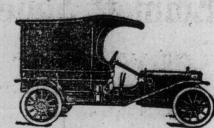
Delivery Waggon-\$6 F. O. B. Windsor. Standard equipment, includes gas lamps and generator, 31x31/2 inch rear tires, shock absorbers in front, three oil lamps, horn and tools.
