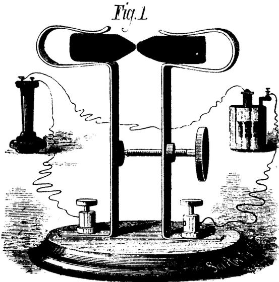
Fig. 1.—A NEW MICRO-TELEPHONE.
