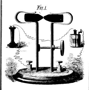
Fig. 1.-A NEW MICRO-TELEPHONE.
