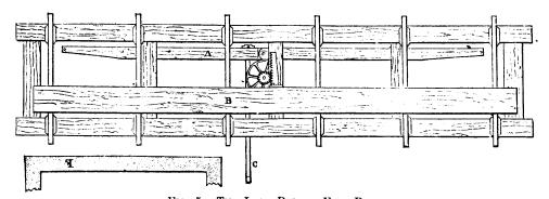
$\begin{tabular}{lll} FIG. 5. -- The Lane-Pottee Foot-Rig.\\ A, jointed foot-var. & B, set-beam. & C, treadle-bar under foor. & D, portion of saw-frame.\\ \end{tabular}$
