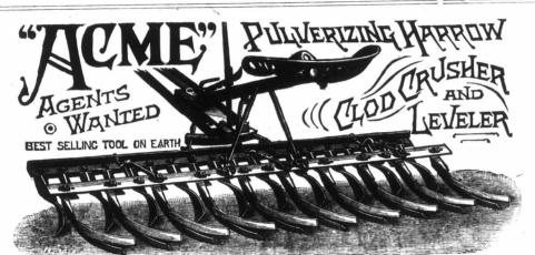
Subjects the soil to the action of a Steel Crusher and Leveler, and to the Cutting, Lifting, Turning Frocess of Double Gangs of Cast Steel Coulters. Immense cutting power. Crushing, Leveling and Pulverizing performed at the same time, Entire absence of Spikes or Spring Teeth avoids pulling up rubbish. Only Harrow that cuts over the entire surface of the ground. Sizes, 3 to 15 feet wide. With and without Sulty attachment. We deliver free at Distributing Depots.
