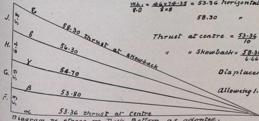
Fig. 3.—Stress Diagram of Dock Bottom; Fifteen Feet Thick at Centre.
