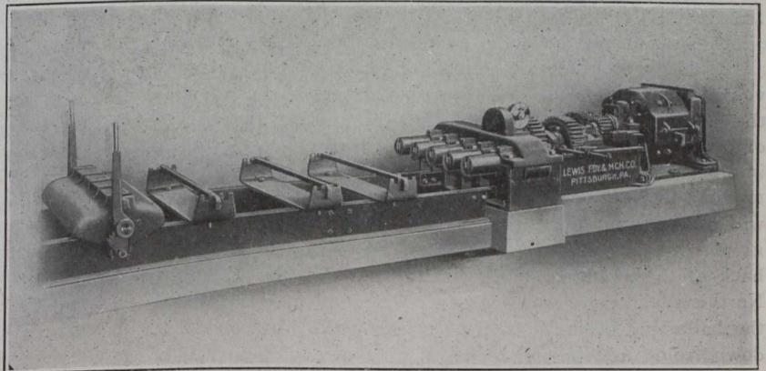
the twisting process, which usually results in an inferior product due to the elastic limit of the bar being exceeded. With a motor gear-connected to the machine, as shown in the accompanying illustration, an occurrence of this kind is practically impossible, since this method of motor connection insures constant torque being applied during the time the bars are being twisted.
