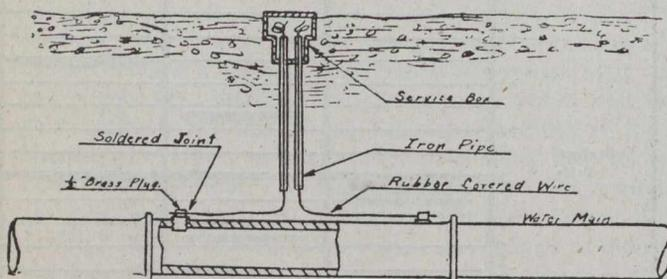
Fig. 5.—Permanent Electrical Test Wire from Surface of Street to Pipe.
