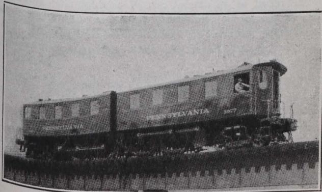
Fig. 2.—A Pennsylvania Railroad 160-ton D.C. Locomotive (600 Volts) for New York City Pennsylvania Terminal Operation.
