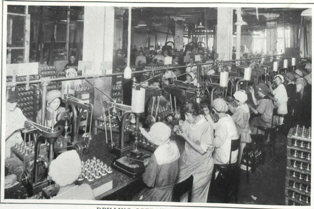
DRILLING OPERATIONS ON BODY
