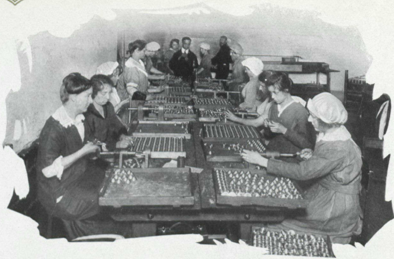
SIZING SET SCREW HOLES AND THREADING CAPS
