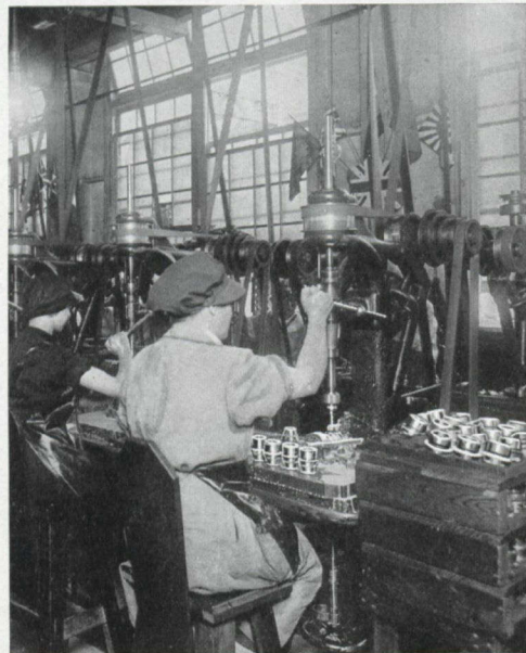
CLOSE-UP VIEW DRILLS FOR CENTRIFUGAL BOLT HOLES
