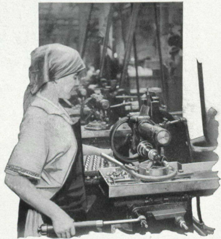
MILLING SCREW DRIVER SLOT IN CAP
