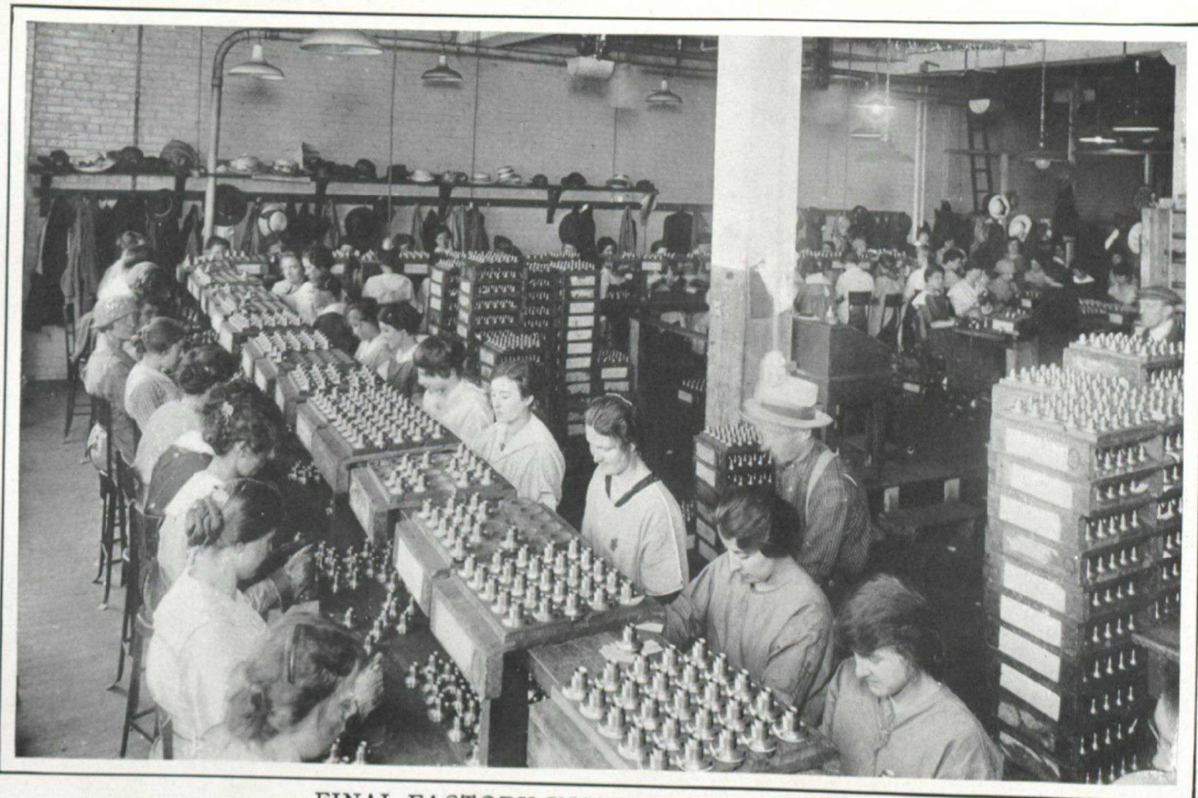
FINAL FACTORY INSPECTION OF BODIES
