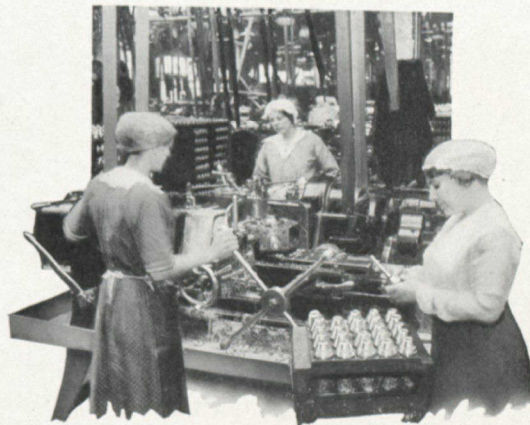
INDIVIDUAL VIEW SHAVING AND GROOVING BODY
