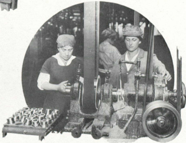
MILLING THREAD ON OUTSIDE OF BODY
