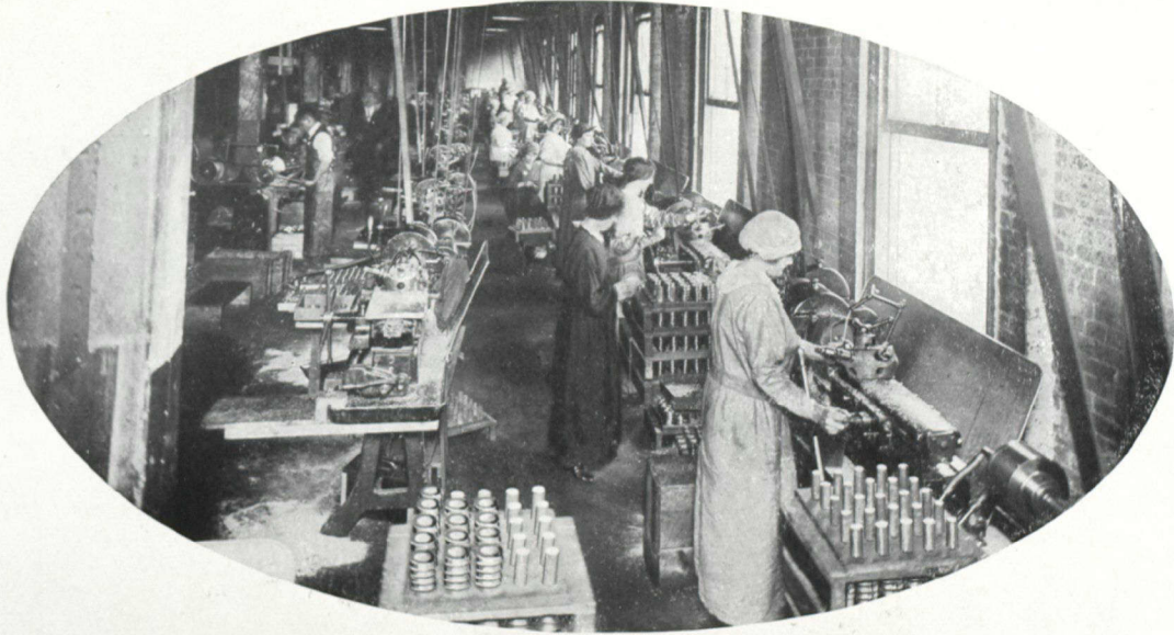
VIEW OF DEPARTMENT FOR BORING AND FACING TIME RINGS
