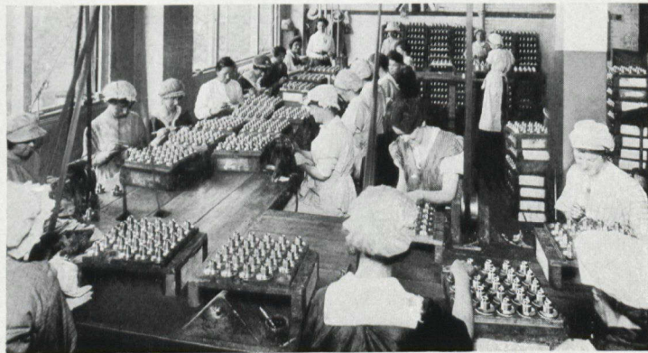
ENAMELLING GRADUATIONS ON THE BODY
