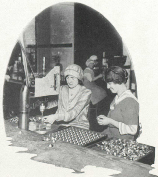
THREADING SET SCREW HOLES
