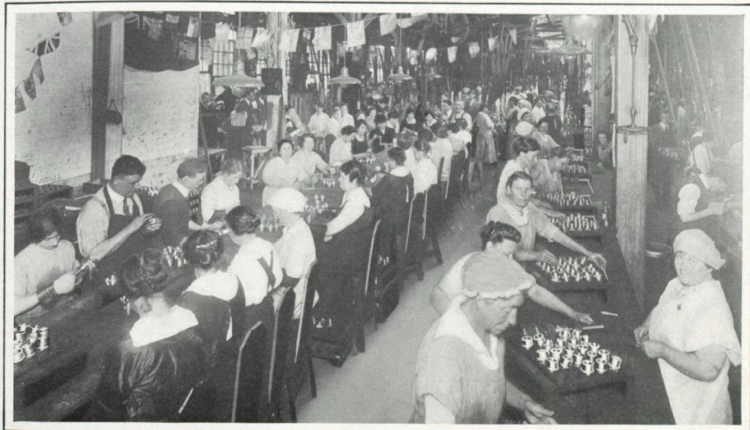
BURRING AND FINISHING BODIES BEFORE PLATING
