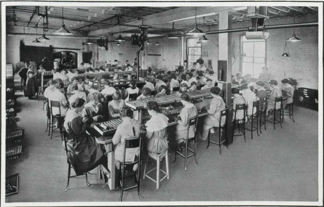
FACTORY INSPECTION OF TIME RINGS, CAPS AND BASE PLUGS
