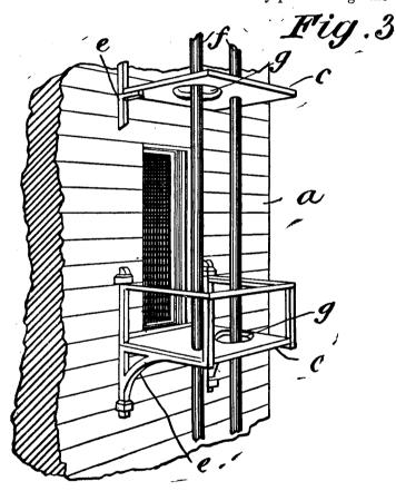
floors or staging from the root to the ground; g g are circular openings which alternate from one side to the other at each succeeding landing. The landing to be placed before a window at every story.
