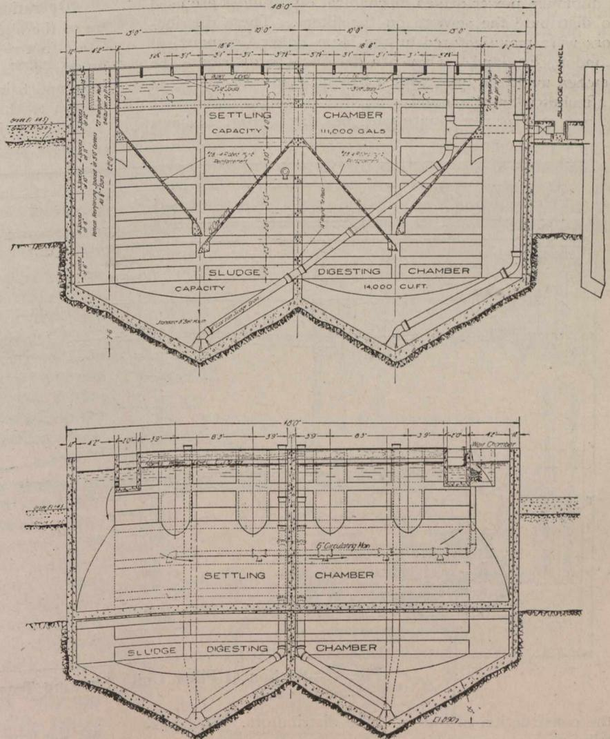
Fig. 3.—Detail Sections of Main Settling Tank.—Upper Section on CC., Lower Section on BB.
