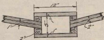
UNDERDRAINAGE AND TIMBER FOUNDATION FOR AQUEDUCT
