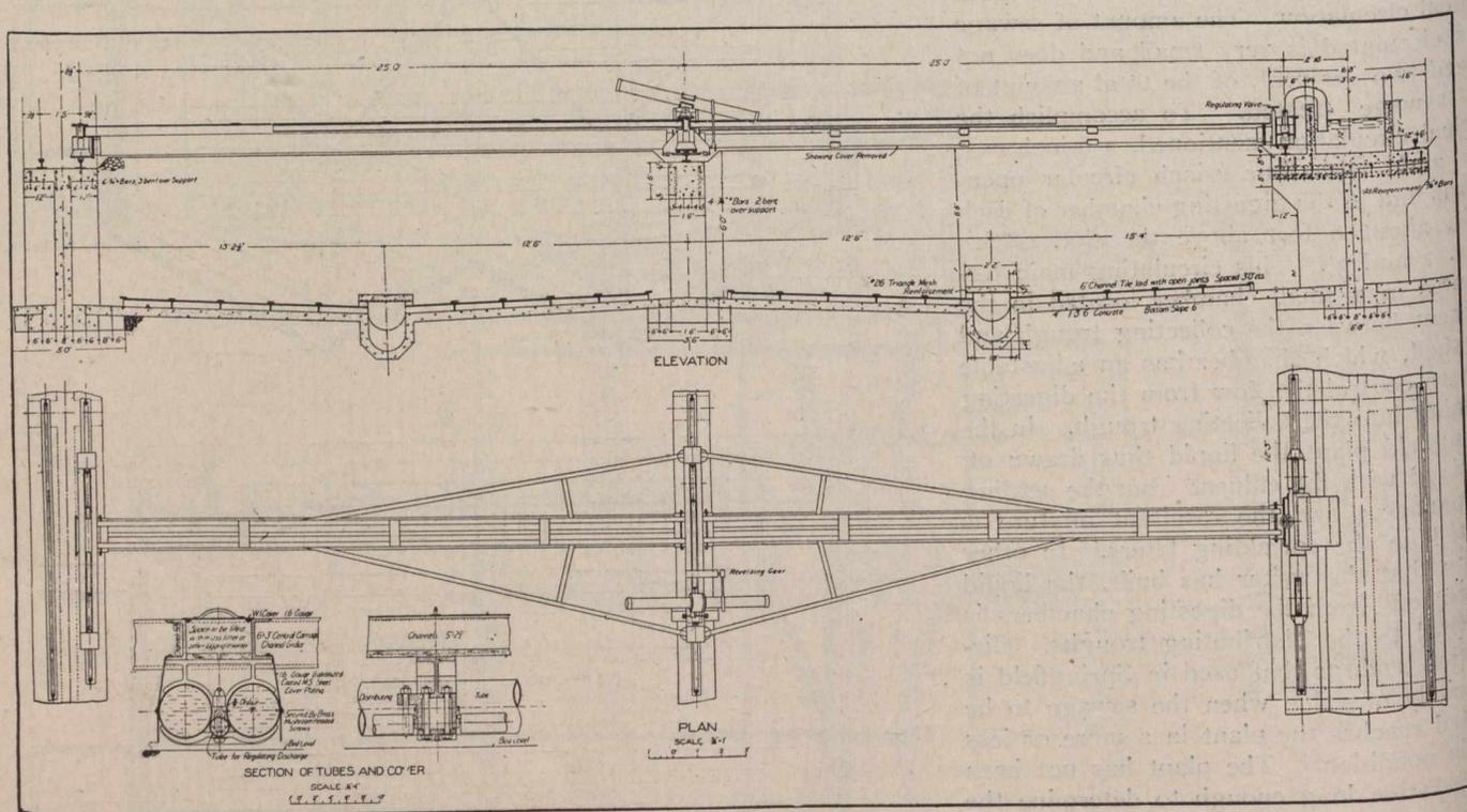
Fig. 4.—Section of Filter Unit Showing Traveling Distributor.
