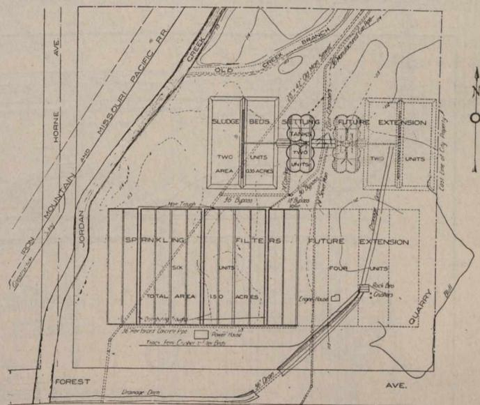
**Fig. 1.—Location Plan of Southern Sewage Disposal Plant.**
