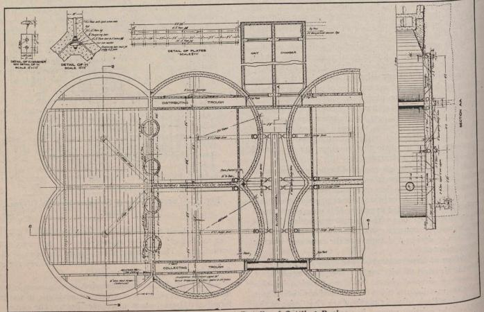
Fig. 2.-Plan and Details of Settling Basins.
