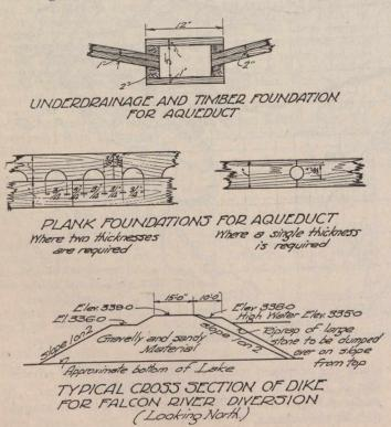
Fig. 3.—Details of Aqueduct Foundation, and Section of Falcon River Embankment.
