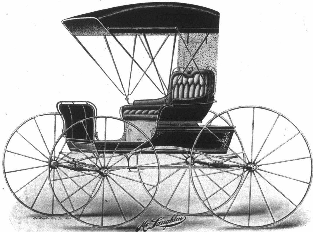
No. 10.—McLAUGHLIN GEAR. FANCY DECORATED CORNING BODY. Fancy Trimmings, deep Wings on Cushion. Part plated top Braces. Plated Brass top Nuts, seat back rail, seat handles, arm rails, dash rail and dust caps. Fancy lining in top with pinked edges. Body and seat handsomely decorated. See No. 1 on page 9 for other specifications.
