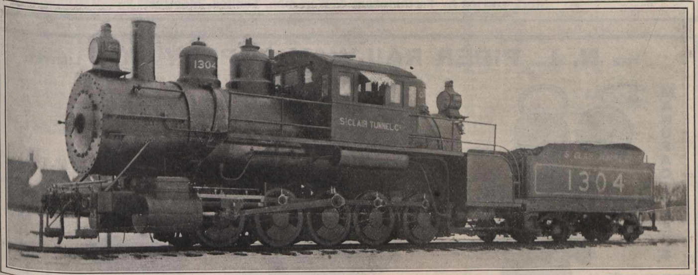
ONE OF THE STEAM LOCOMOTIVES USED IN THE ST. CLAIR TUNNEL PRIOR TO ITS ELECTRIFICATION
