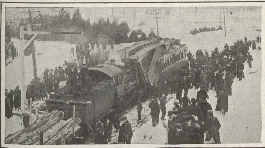
An Unusual Railway Accident Which Occurred near Ottawa Recently. A Passenger Train Was Backing Up and Was Struck by a Freight. Two Passenger Cars Were Telescoped. Photograph by Pittaway.
