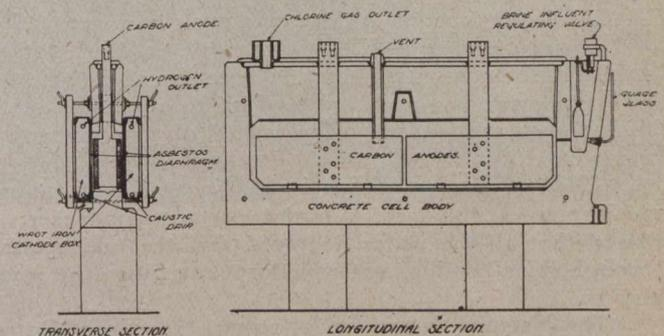
Detail of Cell, Electrolytic Chlorine Plant.
