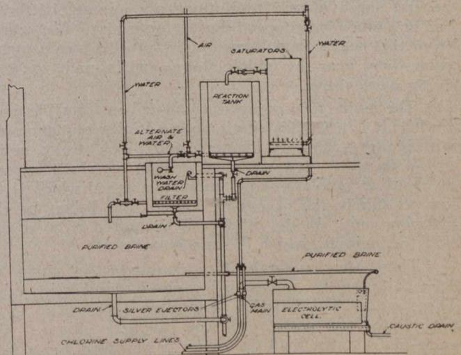
Sectional Elevation Showing Brine Purifying Apparatus and Electrolytic Cell
