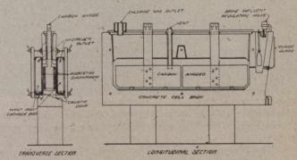
Detail of Cell, Electrolytic Chlorine Plant.
