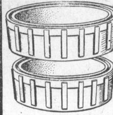
The "Sunshine" has a straight-sided semi-steel firepot, extra heavily ribbed and made in two sections. The two sections allow for contraction and expansion—which prevents cracking. The heavy ribs and semi-steel give extra strength and added radiating surface. Ashes cannot adhere to the straight sides which assures an all-over clear fire. This means the greatest heat from the fuel consumed.
