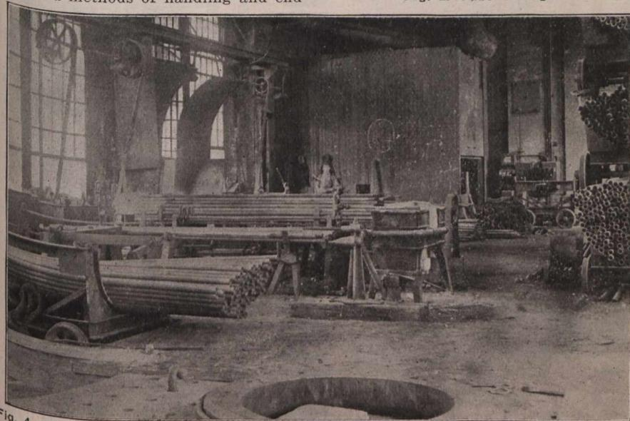
Fig. 4. Department where the Tubes are trimmed, New Ends welded on, and finally cut to Length.
