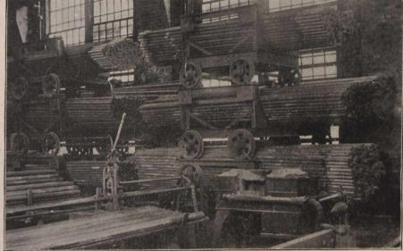
Fig. 2. Tube Storage in Rack Cars specially constructed for the Purpose.
