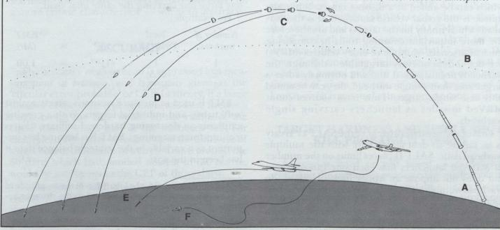
They re-enter the atmosphere and travel a course determined by the initial thrust and the force of gravity. A *cruise* missile is an air-breathing missile which is propelled by a jet engine and never leaves the earth's atmosphere. Other missiles such as the short-range attack missile (SRAM) also operate within the atmosphere.
