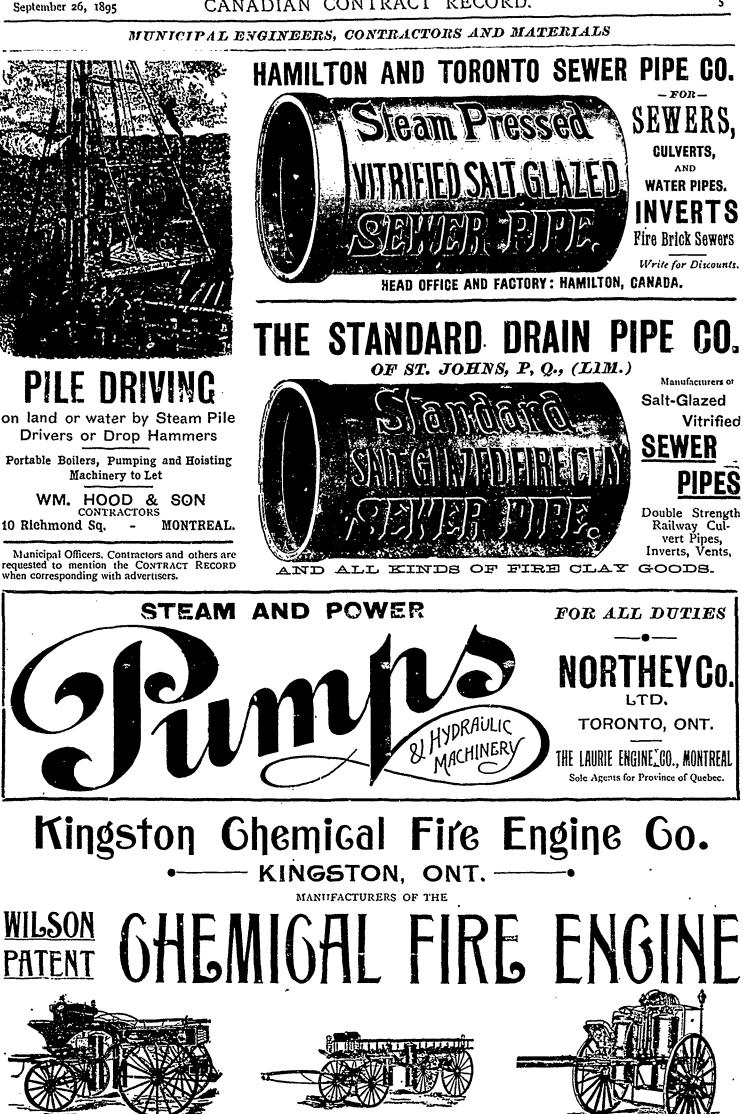
This machine is the most powerful fire fighter. It has two cylinders, 40 gallons capacity each. The combination of chemicals will not freeze, renders material with which it comes in contact non-inflammable, and will not corrode when not in use. For full particulars, write to the Head Office of the Company at Kingston.
