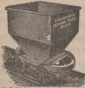
69—R. H.'s Improved Steel Hopper Wagon with Slide Door
