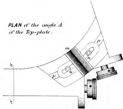
The V shaped groove m and the plate n are cast in one piece and are moveable along a slot in p.
