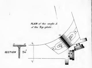
The V shaped groove m and the plate n are cast in one piece and are moveable along a slot in p.
