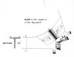
The V shaped greeve m and the plate n are east in one piece and are moveable along a slot in p.
