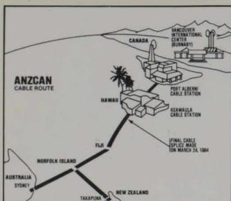
The 15 000-kilometre ANZCAN undersea cable, one of the largest telecommunications projects of its kind, is at present capable of carrying 1 380 simultaneous telephone conversations on the one copper and steel conductor. This is made possible by using a technique known as 'multiplexing' which enables more than one signal to be carried on the same transmission path.
