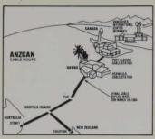
The 15000-kilometre ANZCAN undersea cable, one of the largest telecommunications projects of its kind, is at present capable of carrying 1380 simultaneous telephone conversations on the one copper and steel conductor. This is made possible by using a technique known as 'multiplexing' which enables more than one signal to be carried on the same transmission path.
