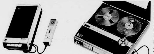
Features: • New Servo controlled motor electronically and automatically corrects for speed variations and maintains precise timing accuracy . SONY-O-MATIC - completely automatic recording volume control (manual control possible if desired) • Advanced Solid state circuit • House current, flashlight battery or optional rechargeable battery operation • Dual track, two speeds (3 <sup>3</sup>/<sub>4</sub> ips & 1 <sup>7</sup>/<sub>8</sub> ips), full 5-inch reel capacity (plays with lid closed)
