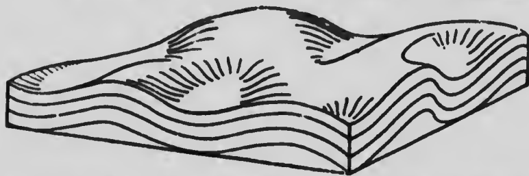
FIG. 2.—View of a part of the earth's crust formed of stratified rocks, which have been thrown into waves, producing synclinal hollows and anticlinal upfolds. The anticlines and synclines seen on the sides of the block are evidently due to cross-sections of dimples and bulges on the surface. In nature, the surface is of course modified by denudation.
