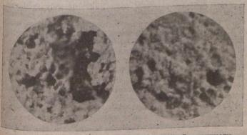
"NORMAL" CONSISTENCY FIG. 1—TEXTURE OF CEMENT MATRIX IN CONCRETE OF DIFFERENT CONSISTENCY (X 60)
