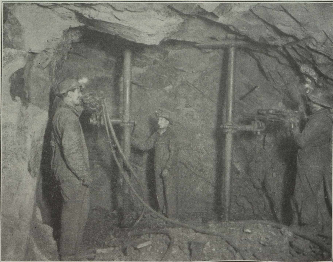
Drifting in Creighton Nickel-Copper Mine, Sudbury District Ontario.—Mining Nickel-Copper Ore in a Canadian Mine.
