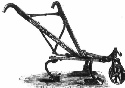
Arranged with Turnip Blades for Flat Cultivating.
