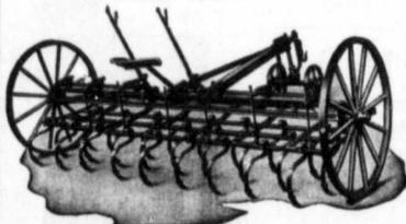
Can be fitted with wide points for shallow cultivation, if desired.
