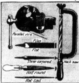
thing for a beginner to remember is that a file cuts only on the forward stroke, like a saw, and that therefore the pressure on the return stroke must not be heavier than will just keep the file on the work. The working strokes should be steady and with an even pressure from tip to heel of the file. The man who merely
