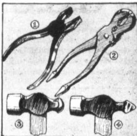
individually; but where there are a number together—as in the main bearings and big-ends of an engine that is being dismantled—it saves time to go about the job as follows: First close all the tails with a punch and light hammer, and with the hammer drive the pins out a little so that their heads project from the nut, then take the pliers and wrench them out.
