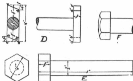
of cast iron and quite heavy; steel dies are provided for bolts of different sizes, usually varying by 1/8-inch, although occasionally 7-16th-inch and 9-16th-inch dies are used. The length of the bolt is determined by a steel block (a) provided with notches that engage a series of notches on the
