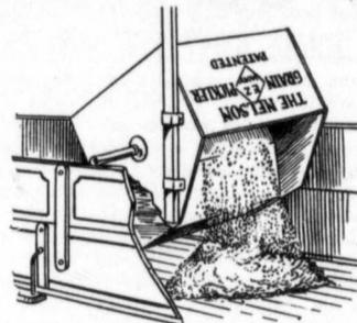
No. 3 Position—Showing Grain Being Dumped
