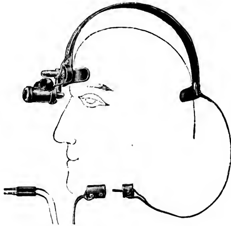
Fig. 6.—Phillips's electric photophone, with adjustment for focusing light.
