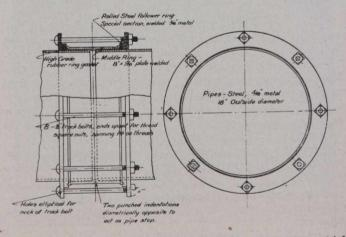
that used on an ordinary piston rod. The Custer joint, which was adopted on the Moose Jaw water supply, compresses the rubber gasket in a different way, and gives some latitude for variations in the size of pipe and couplings. It is stated that hundreds of these joints were made on the Moose Jaw work in a foot or more of water. The accompanying sketch gives a clear idea of the joint.
