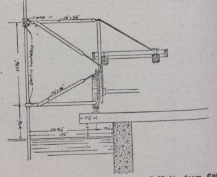
Sketch Showing Method of Suspension of Meter from Car.
