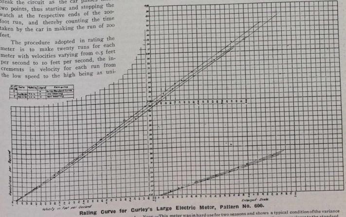
Showing revolutions per second and velocity in feet per second. Note.—This meter was in hard use for two seasons and shows a typical condition of the variance of rating curves. Note that with the old bearing the meter ran fastest, and that the introducing of a new bearing brought the rating curves closer to the standard.
