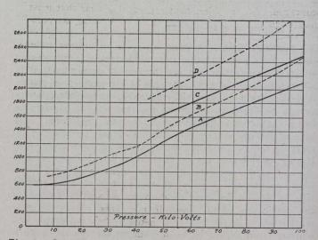
Fig. 2.—Cost in Dollars Per Mile of Transmission Line Complete, Not Including Cost of Conductors, Right-of-Way, and Clearing Cround in Wooded Country.
